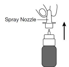
Soak the spray nozzle in warm water and rinse. **Do not** try to unblock the spray nozzle by inserting a pin or other sharp object because this will damage the spray nozzle.
